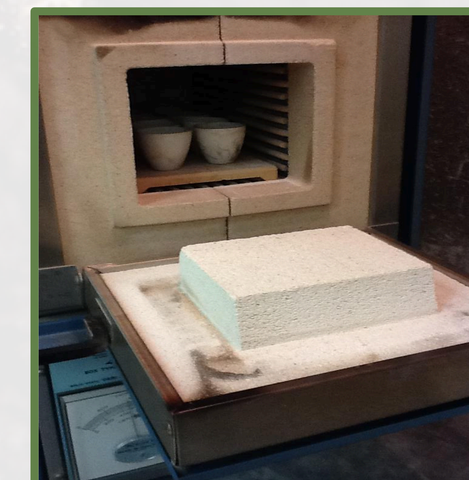
Figure 4: The oven at 500 degrees Celsius when the samples were put into the muffle furnace oven.
